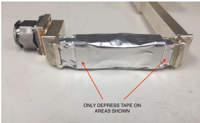
Figure 5 securing the tape in place
