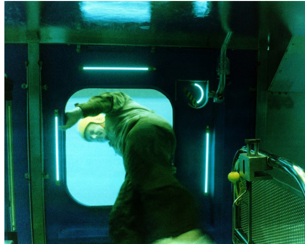
Emergency egress systems, such as this system from Astronics LSI, are required for rotorcraft that fly over water.
