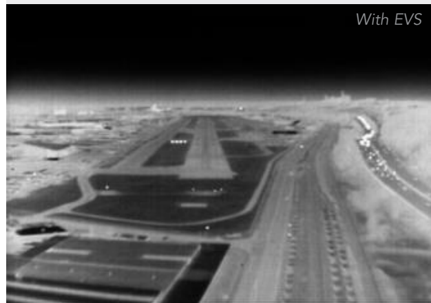
Pilot view of the Boeing Field Airport shown without EVS and then with an EVS system from Astronics Max-Viz.
