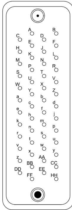
Figure 2-3, Front Panel Connector Pin Numbering
