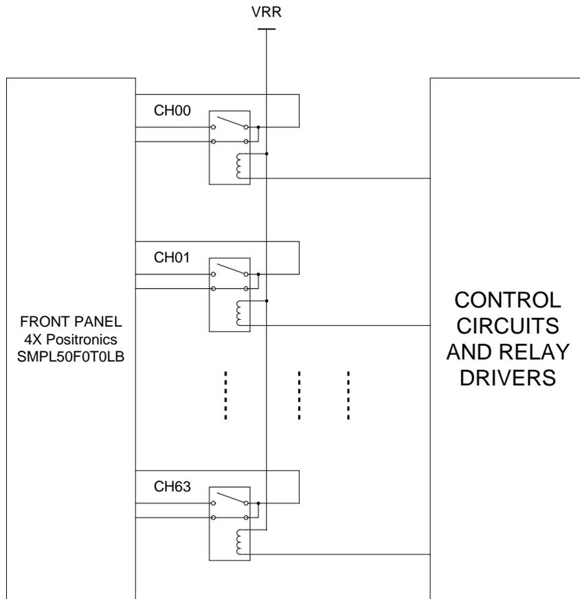
Figure 2-1, 1260-16A, Switch Block Diagram
