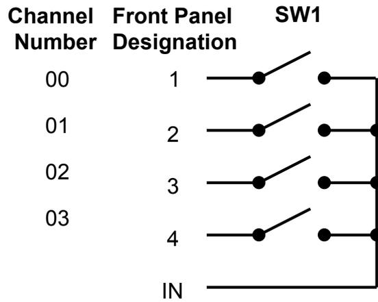
Figure 2-2, 1260-164AH Relay Diagram
