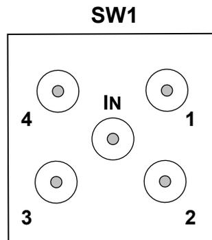
Figure 2-1, 1260-164AH SMA Connector Designations
