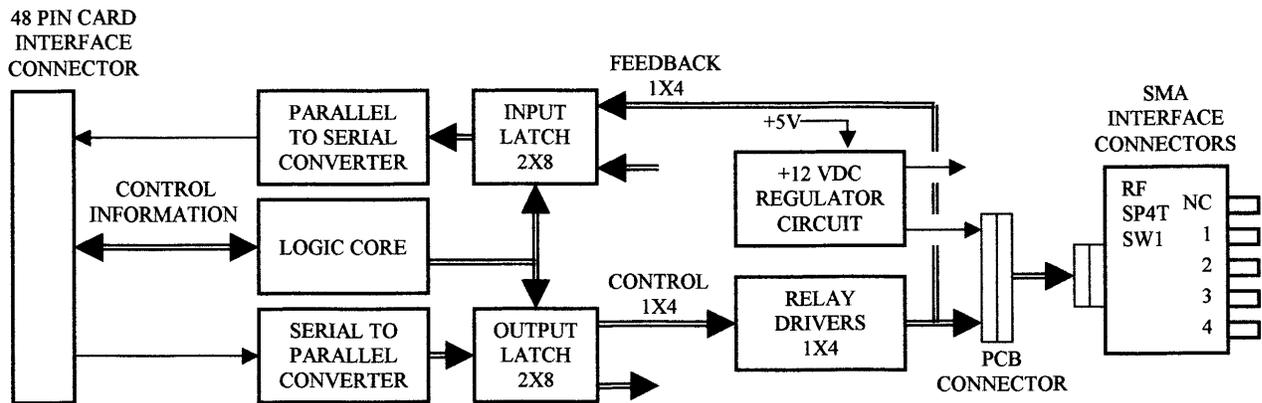
Figure 2-6, 1260-164BH Block Diagram
