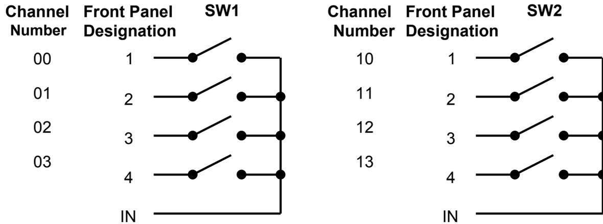
Figure 2-5, 1260-164BH Relay Diagram
