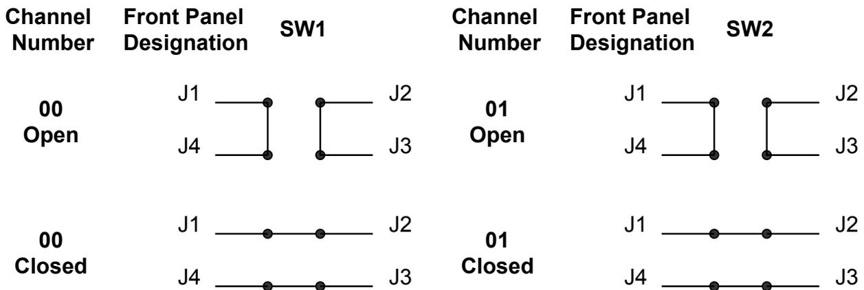
Figure 2-5, 1260-162BH Relay Diagram
