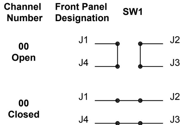
Figure 2-2, 1260-162AH Relay Diagram
