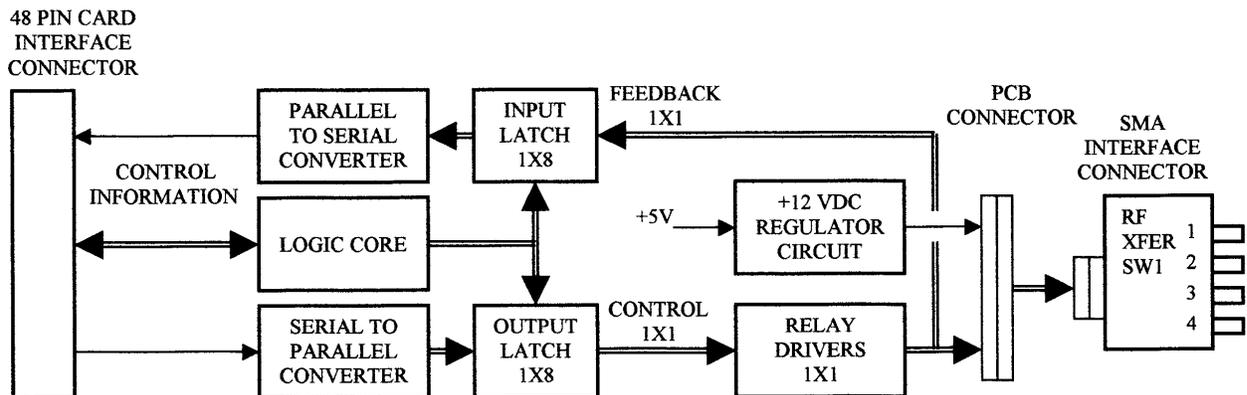
Figure 2-3, 1260-162AH Block Diagram
