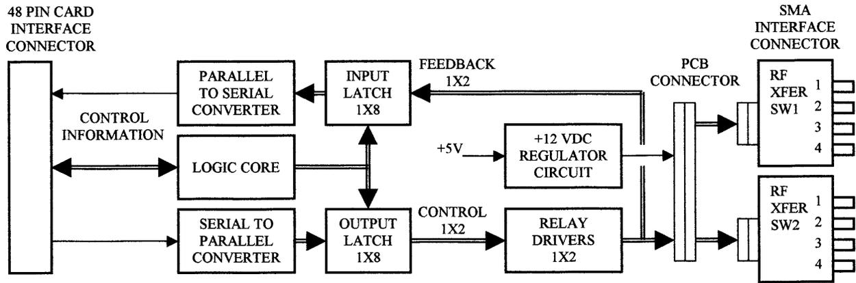
Figure 2-6, 1260-162BH Block Diagram
