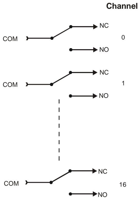
Figure 2-2, Relay Diagram
