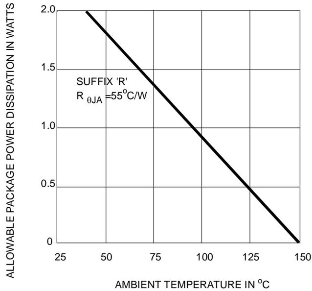
Figure 1-3, Allowable Package Power Dissipation of Output Stage
