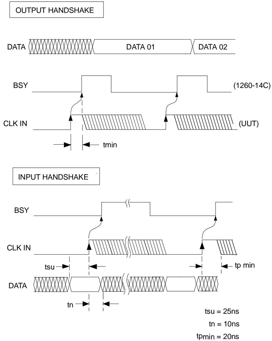
Figure 3-1, 1260-14C Input and Output Handshake Modes
