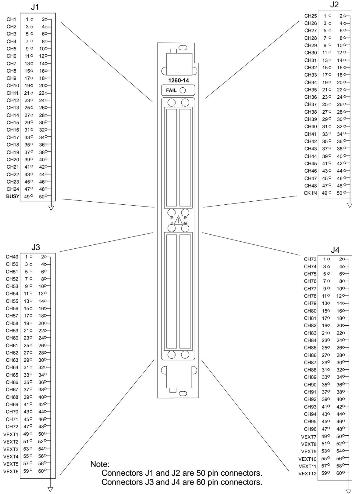
Figure 1-2, 1260-14C Front Panel and Pin Configuration
