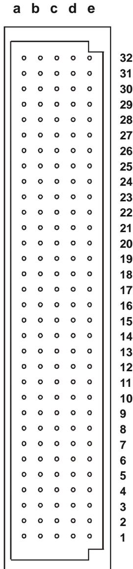
**Figure 2-3, 1260-117A Front-Panel Connector Pin Numbering**
