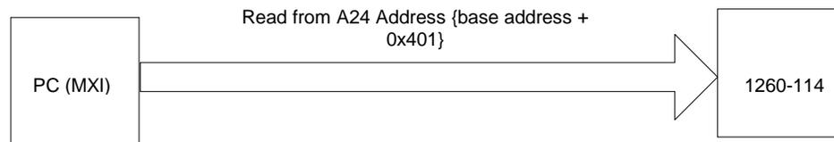
**Figure 3-2, Register-Based Mode of Operation**
