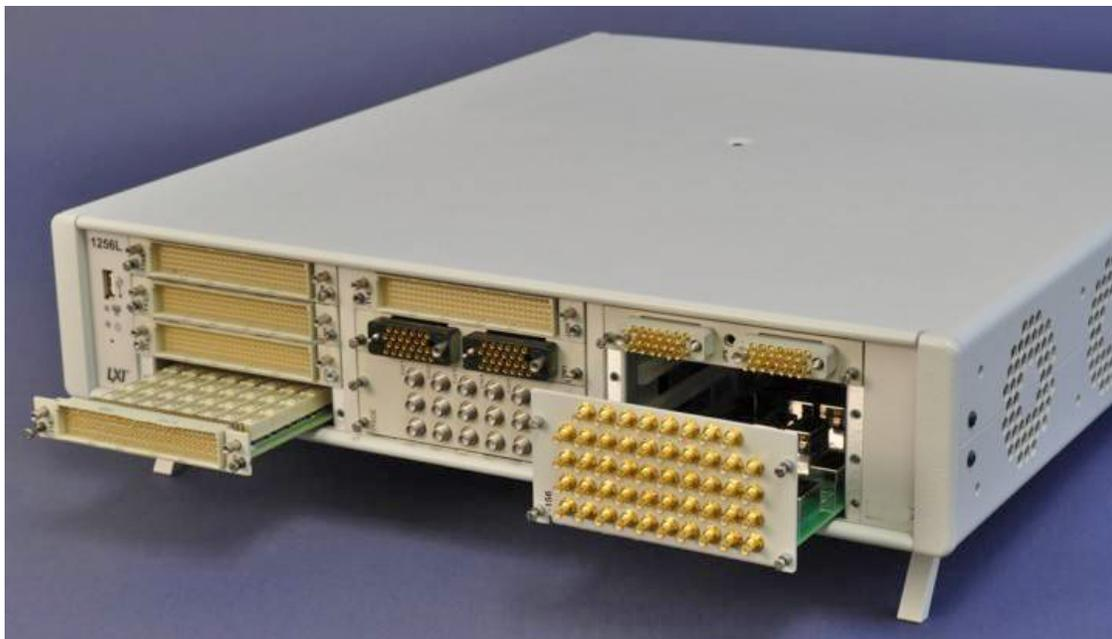
**Figure 1-1, 1256L Switching System (Showing Array of Plug-in Cards)**
