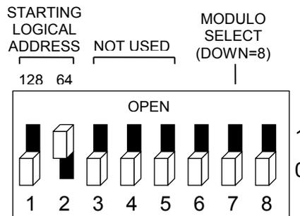
With the above setting, the starting logical address is 64 and the logical addresses are assigned as follows:
