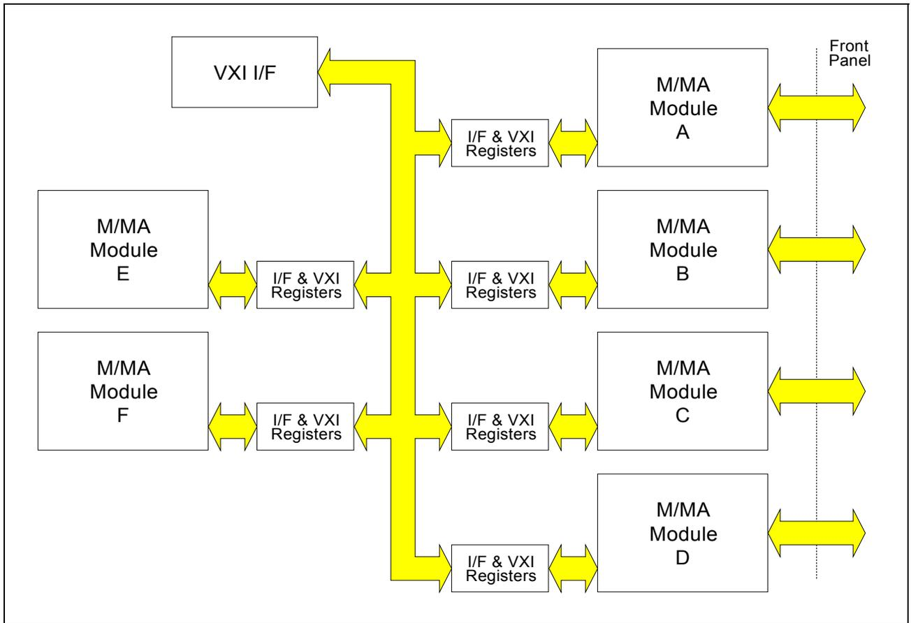
Figure 2-2, VX405C Functional Block Diagram
