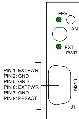
Figure C-1, M213 Front Panel I/O Signals
