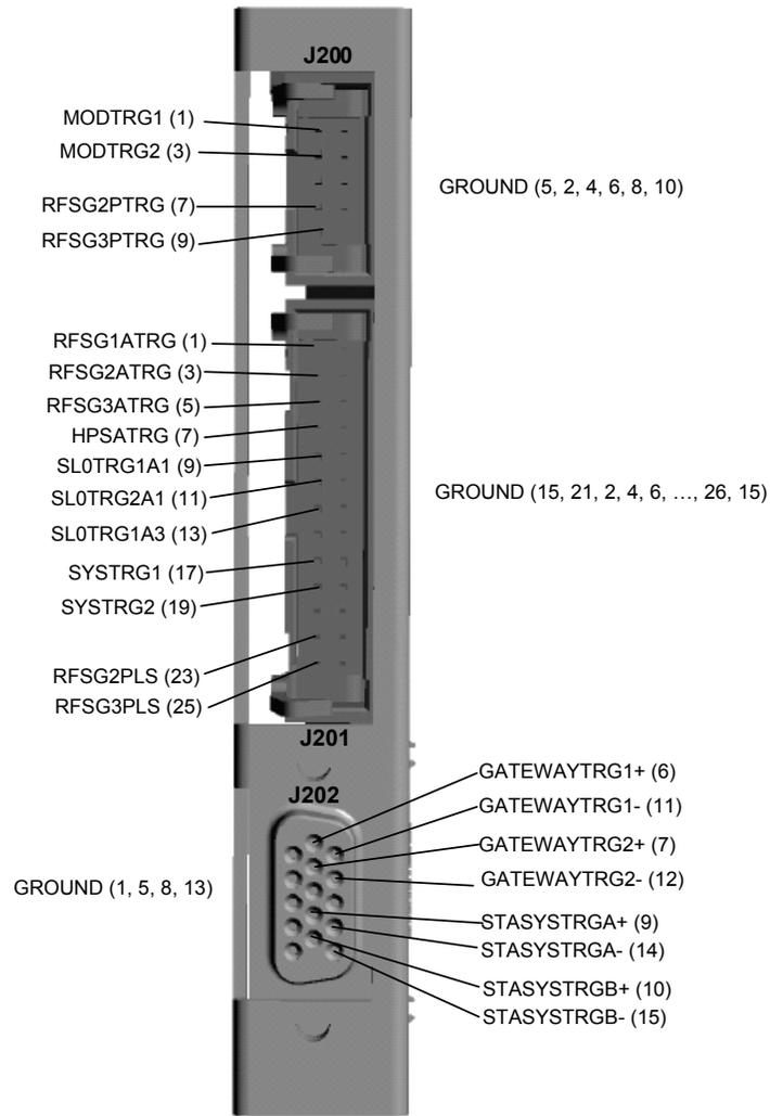
Figure E-1, M1721 Front Panel Connectors
