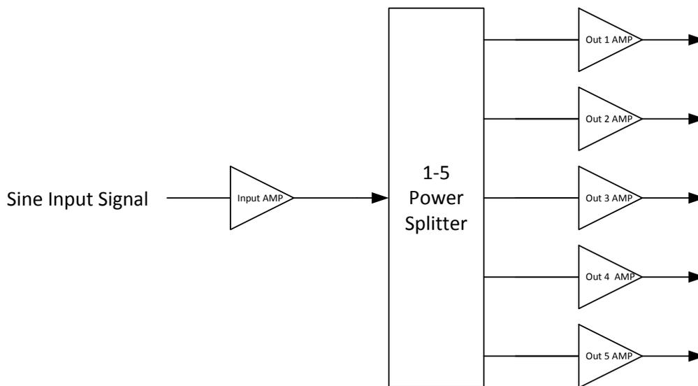
**Figure 5-3, Sine Wave Gain Amplifiers**
