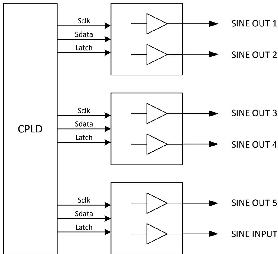
Figure 5-4, Dual Attenuators for Sine Wave Gain Settings
