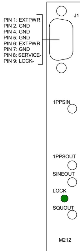
Figure B-1, M212 Front Panel I/O Signals
