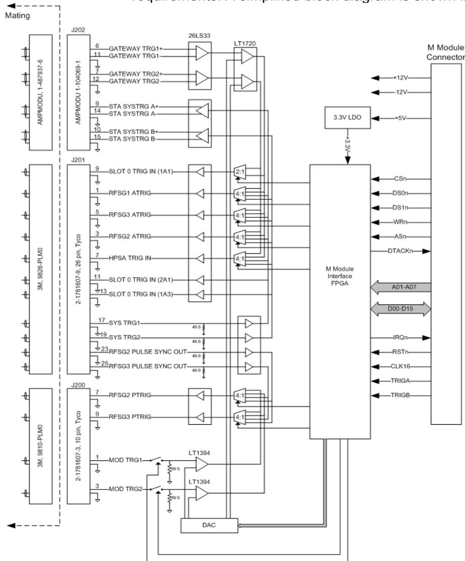
Figure 7-1, Functional Block Diagram
