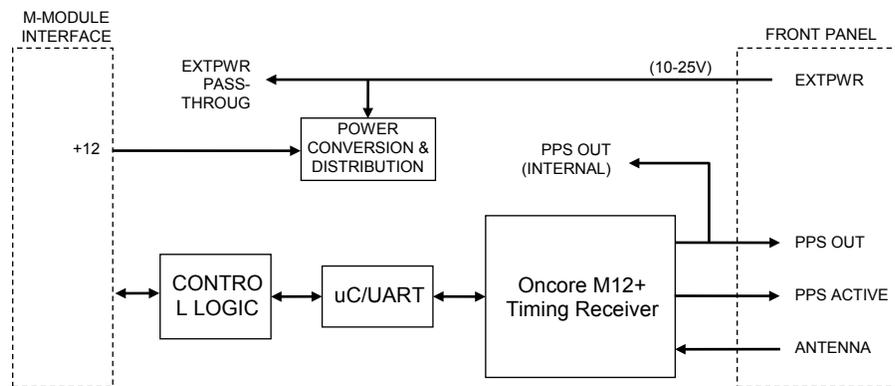
**Figure 4-1, Functional Block Diagram**
