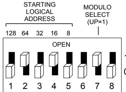
With the above setting, the starting logical address is  $64 + 16 = 80$  and the logical addresses are assigned as follows:
