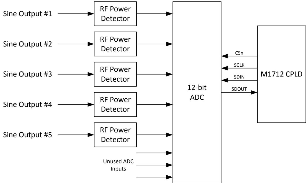
Figure 5-5, Sine Wave RF Power Monitors
