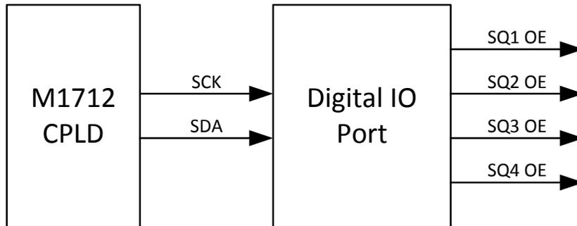
Figure 5-6, Square Wave Output Enable Control
