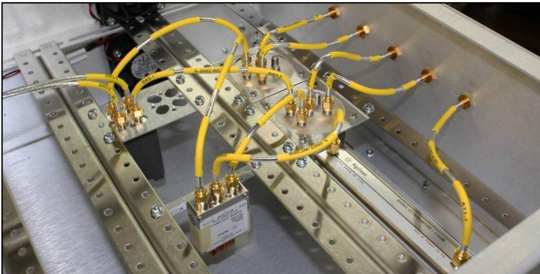
Figure 2-22, 1257A with Components Cabled to a Customized Front Panel (Example)
