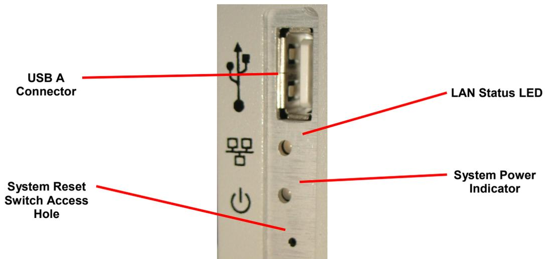
Figure 1-5, 1257A-C Front View Detail
