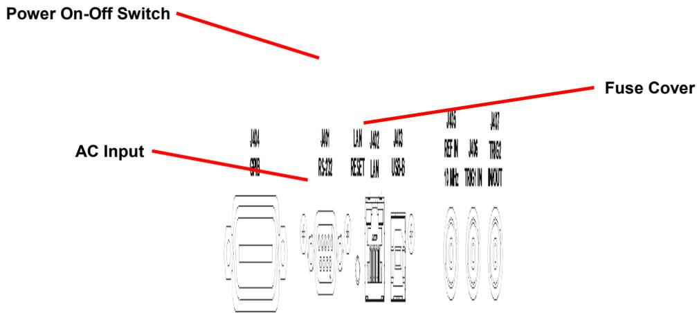
Figure 1-7, 1257A-C 4U Rear View Detail – Upper Area (Appearance Typical)
