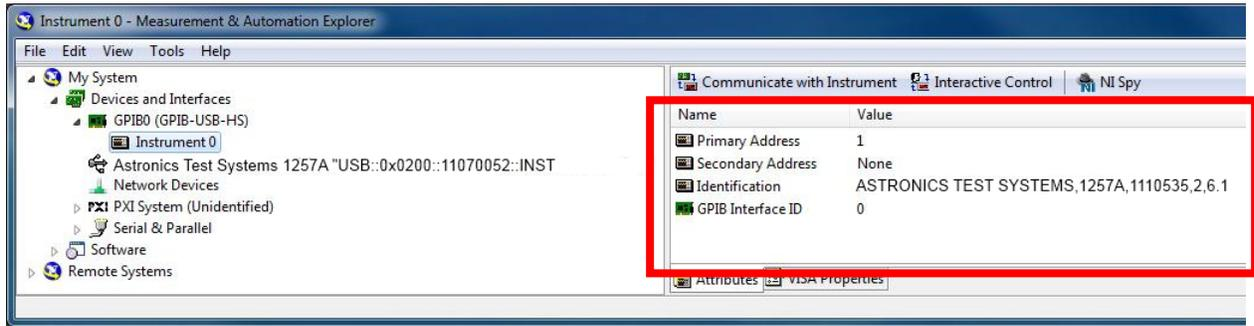
The GPIB VISA resource string for the above device is “GPIB0::1::INSTR”. Note that if there are multiple GPIB interfaces, then the VISA resource string is “GPIB<n>::1::INSTR”, where “n” is the number of the GPIB interface.
