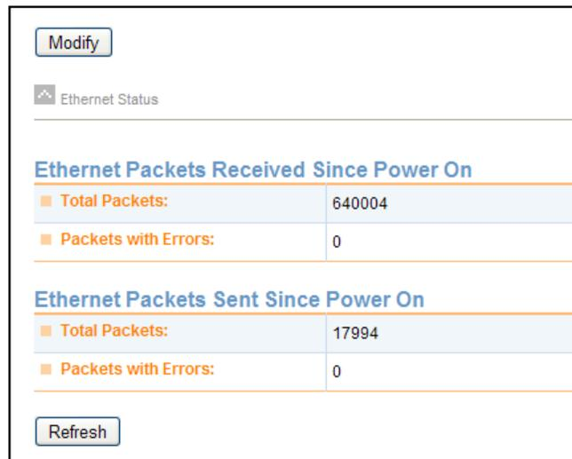
The screenshot shows a web interface for Ethernet Status. At the top left is a 'Modify' button. Below it is the title 'Ethernet Status' with a small icon. The main content is divided into two sections: 'Ethernet Packets Received Since Power On' and 'Ethernet Packets Sent Since Power On'. Each section contains a table with two rows: 'Total Packets' and 'Packets with Errors'. At the bottom is a 'Refresh' button.
