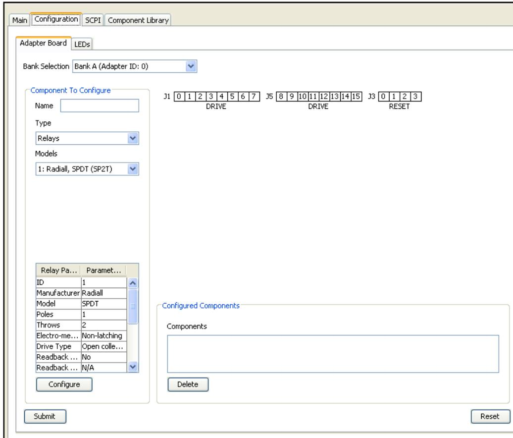
Figure 3-21, Slot Controls/Configuration/Adapter Board Tab (Relay Configuration)
