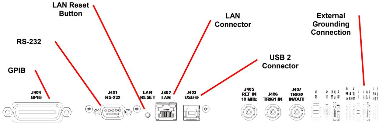
Figure 1-6, 1257A-C 4U Rear View Detail – Lower Area (Appearance Typical)
