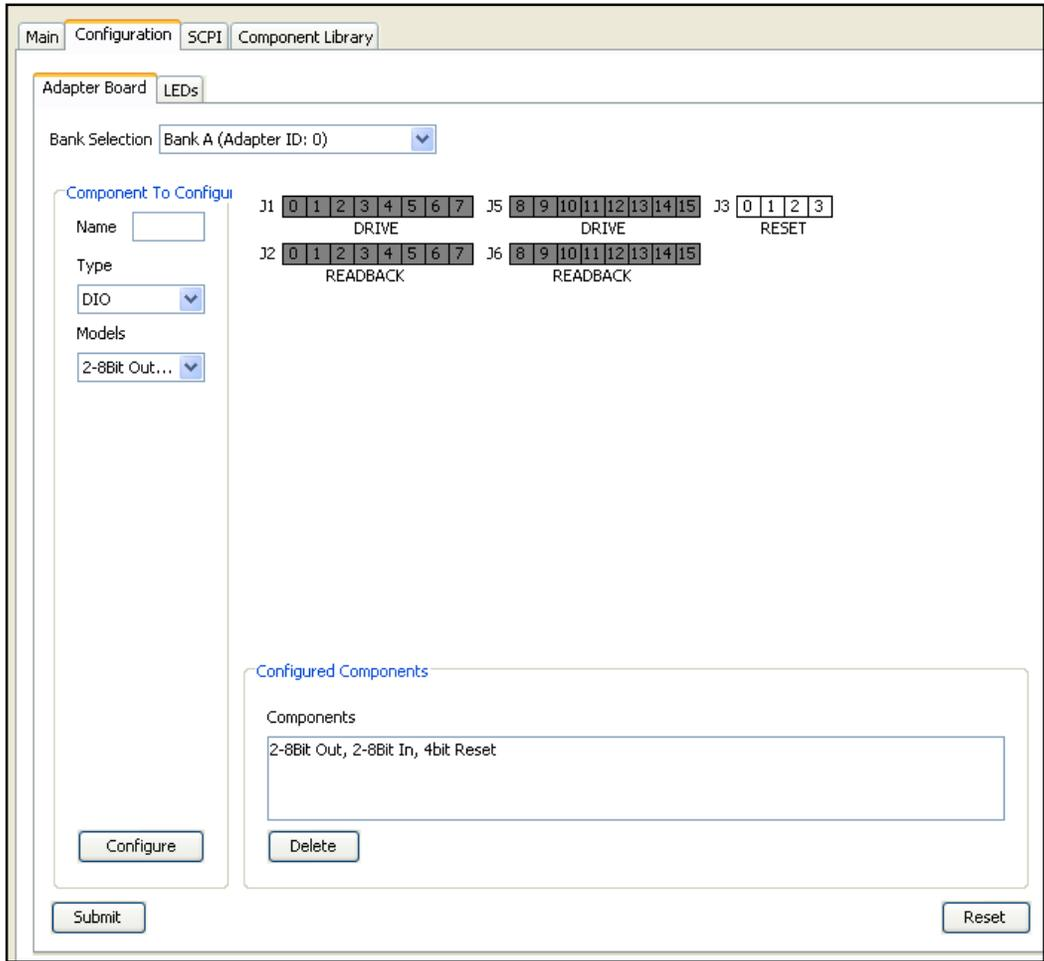
Figure 3-22, Slot Controls/Configuration/Adapter Board Tab (DIO Configuration)
