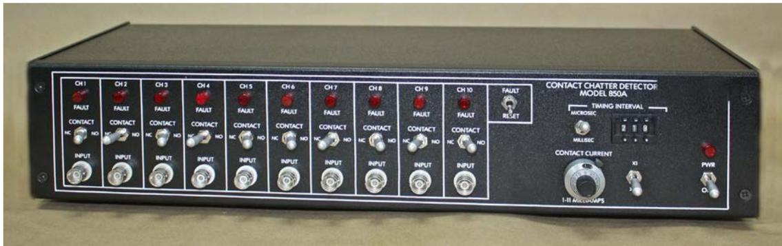
Figure 1-1. Trig-Tek 850A Contact Chatter Detector
