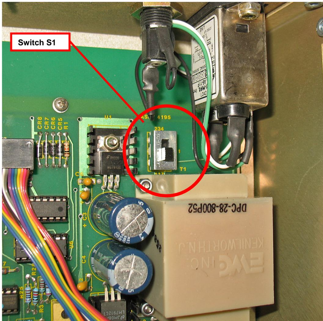
Figure 2-1. Switch S1 – Input Voltage Setting
