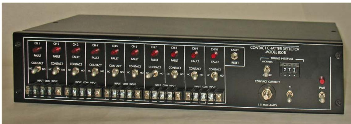
Figure 1-2. Trig-Tek 850B Contact Chatter Detector
