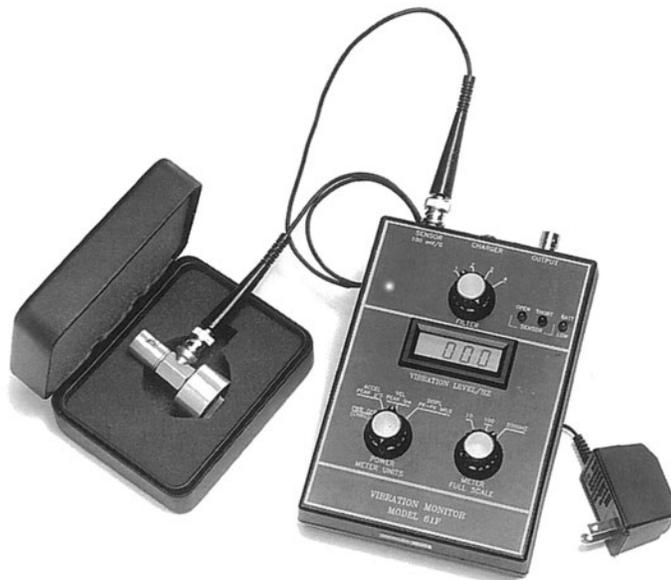
**Figure 1-1, 61-Series Portable Vibration Monitor (61F Shown)**
