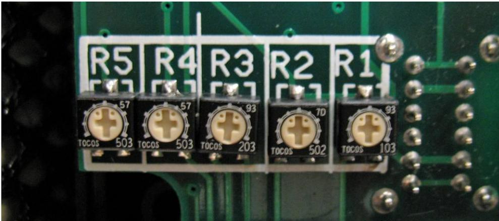
Figure 4-1, Potentiometer Adjustment Locations
