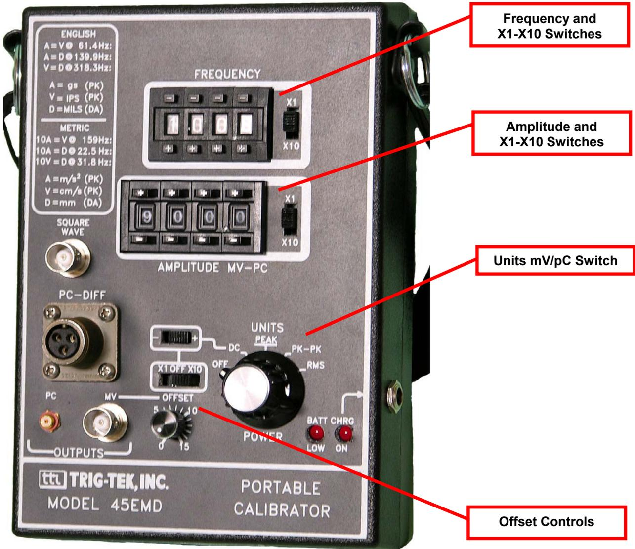
Figure 2-1, 45EMD Control Switches
