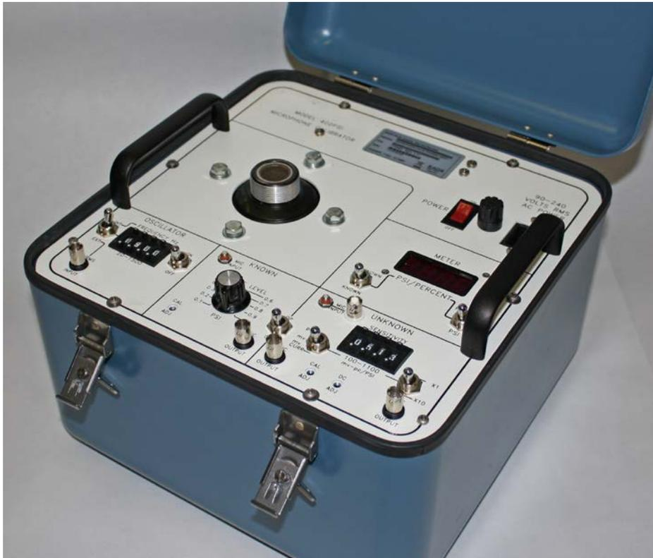
**Figure 1-1, 402 PSI Microphone Calibrator**
