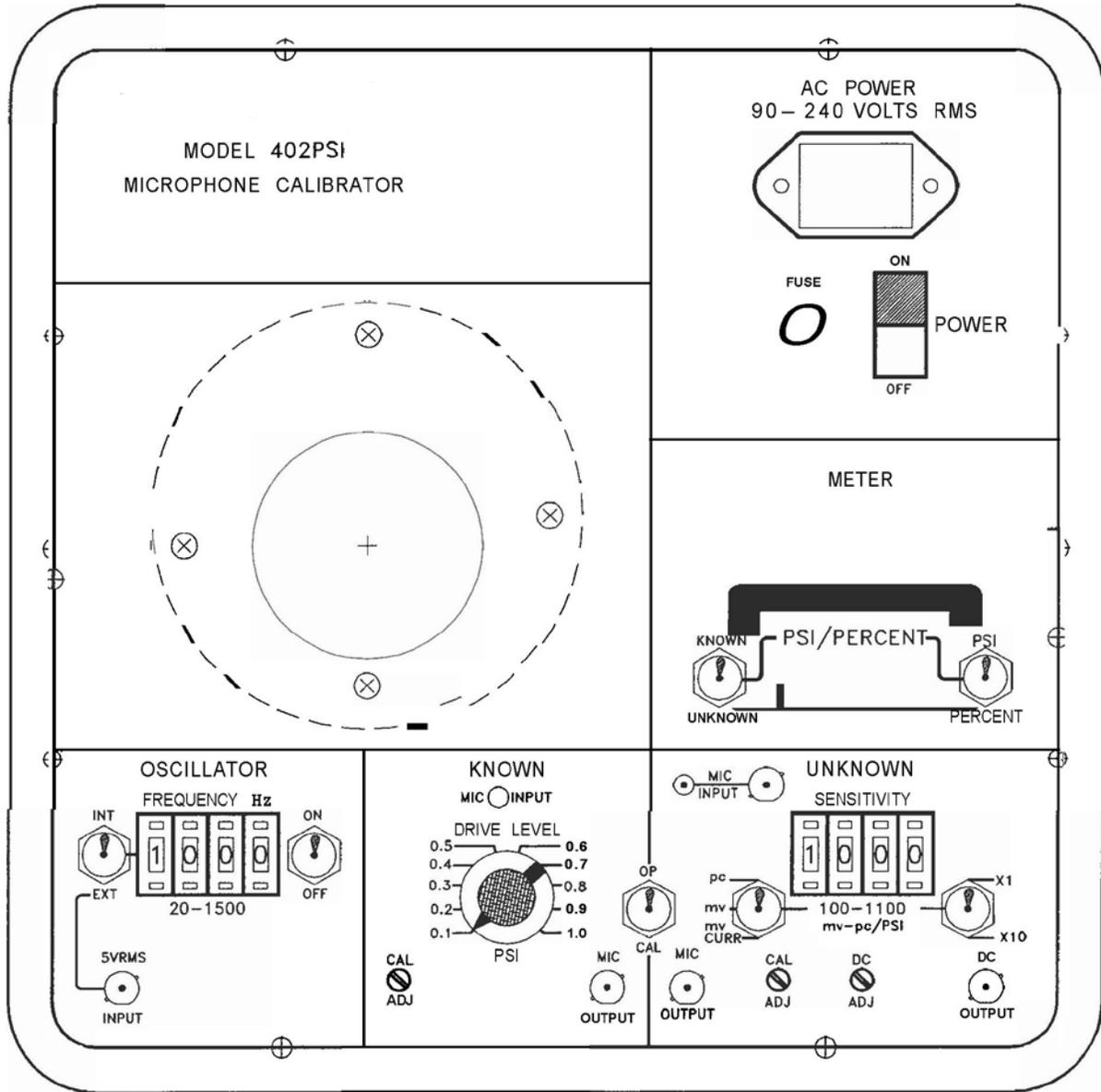
Figure 2-1, 402PSI Microphone Calibrator Front Panel
