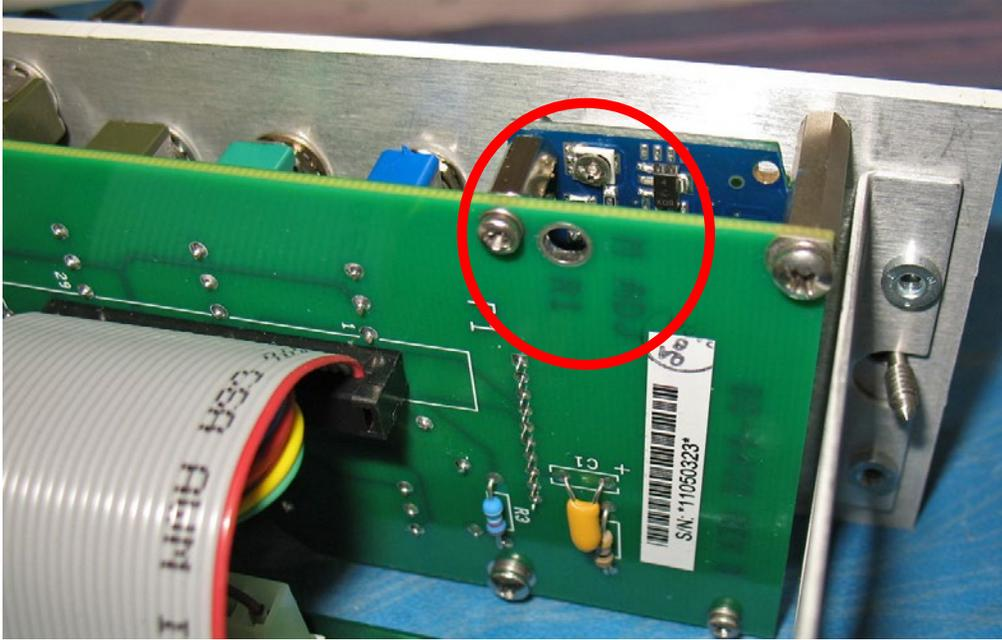
**Figure 4-2, DVM Adjustment Resistor R1**
