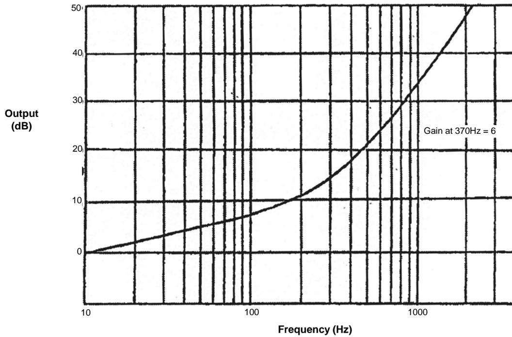
Figure 3-4, Filter 3 Equalizer Frequency Response
