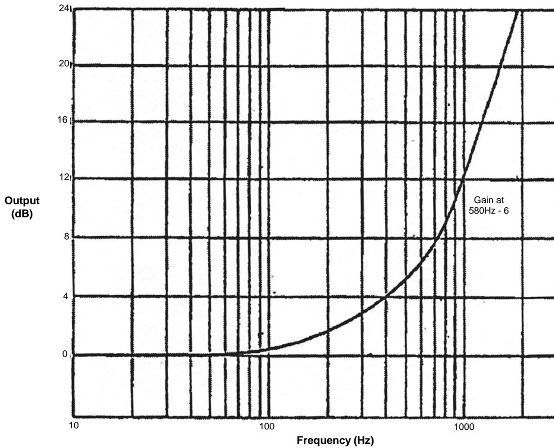
Figure 3-2, Filter 1 Equalizer Frequency Response
