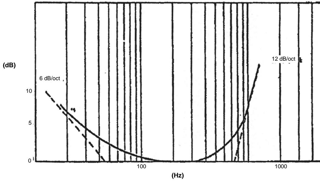
Figure 3-3, Filter 2 Equalizer Frequency Response
