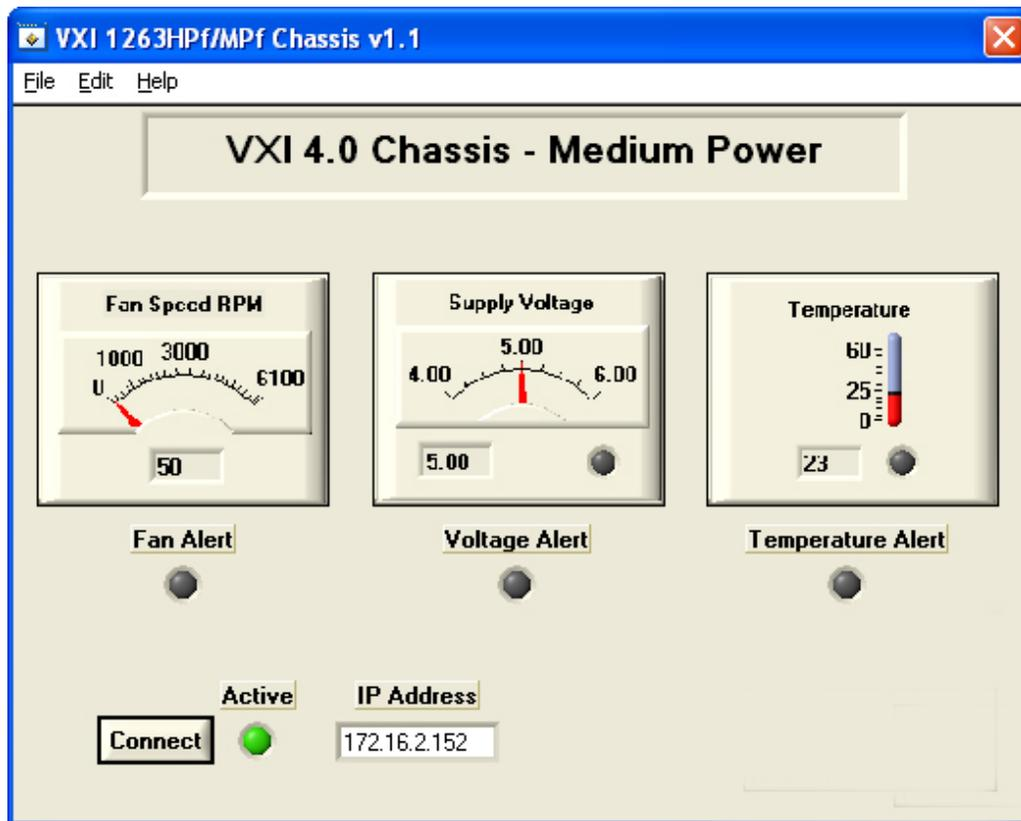
Figure 6-1, Main Monitoring Panel
