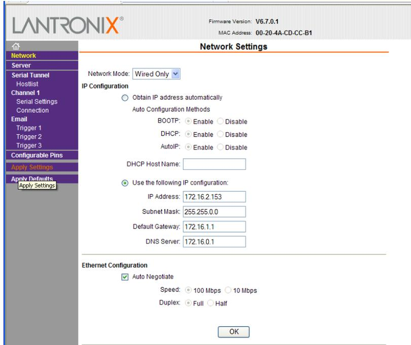
9. After a few seconds, the web page will indicate that the configuration is being saved and the unit will reboot.
