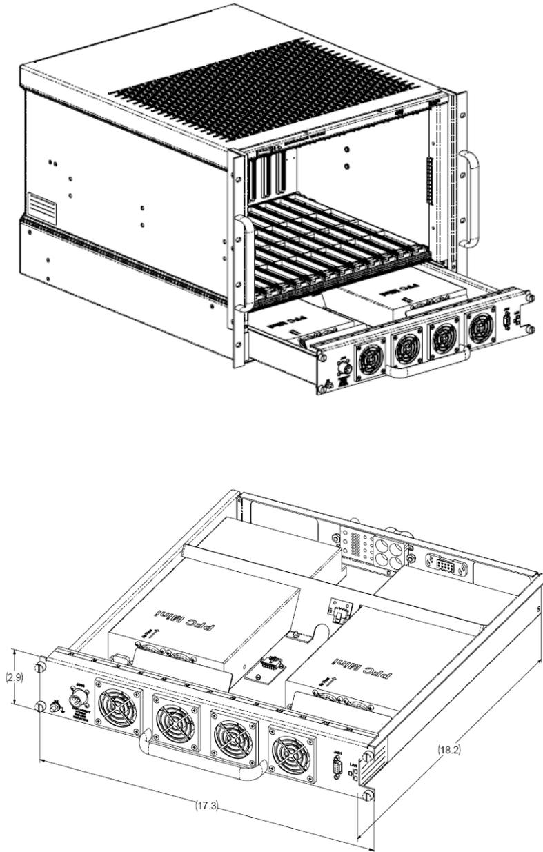
Figure 5-1, Module Power/Fan Assembly Detail
