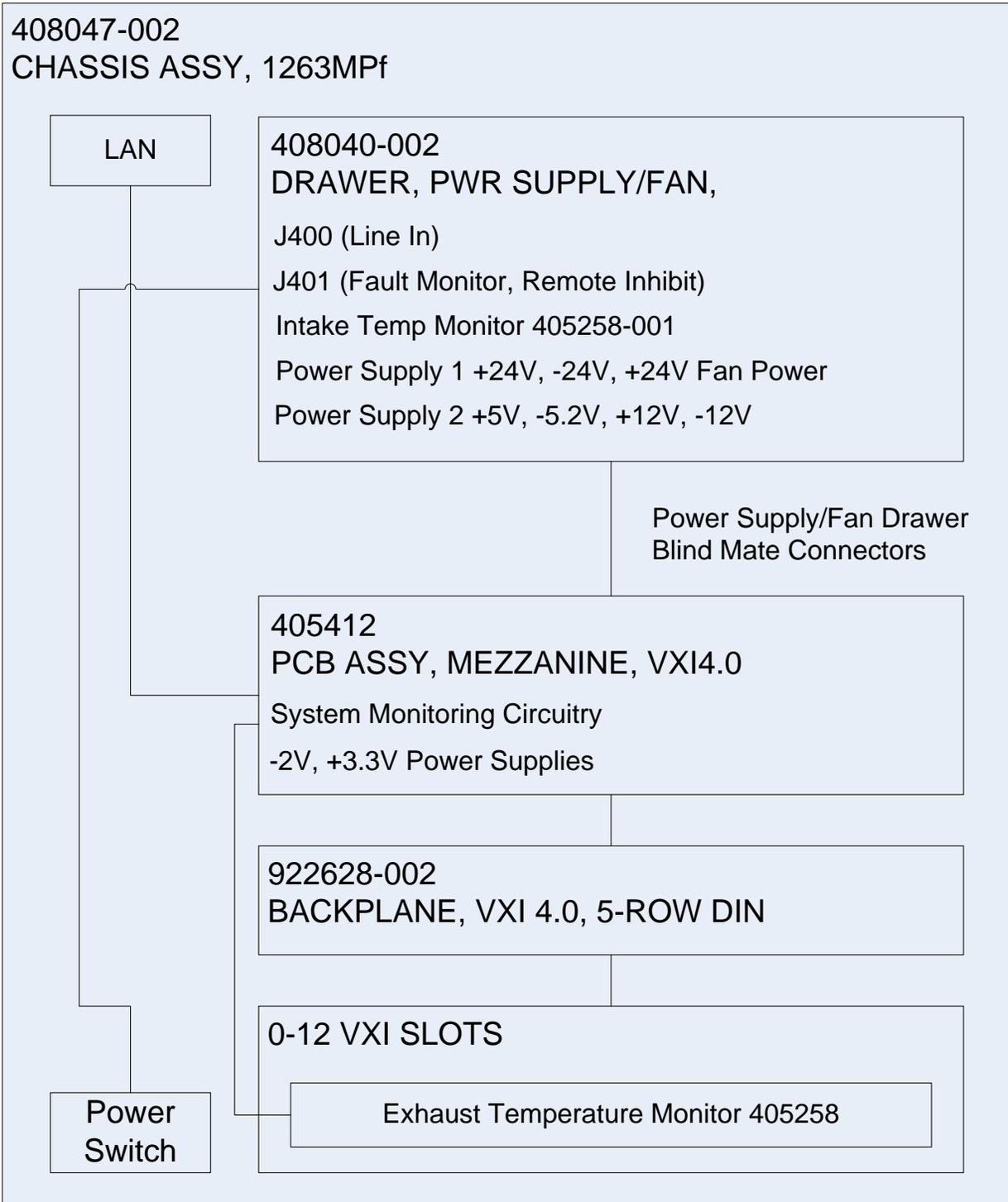
Figure 4-1, 1263MPf Chassis Functional Block Diagram
