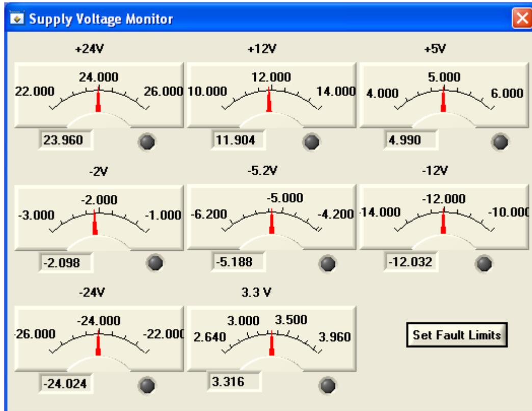
Figure 6-3, Per VXI Rail Voltage Monitoring
