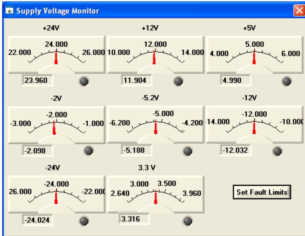
Set Fault limits can be changed as the application requires. Updated or changed settings can be saved on the top SFP under File -> Save Setting as Default.
