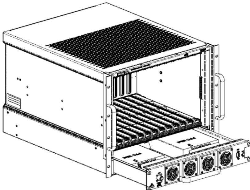
Figure 1-1, 1263MPf VXIbus Mainframe
