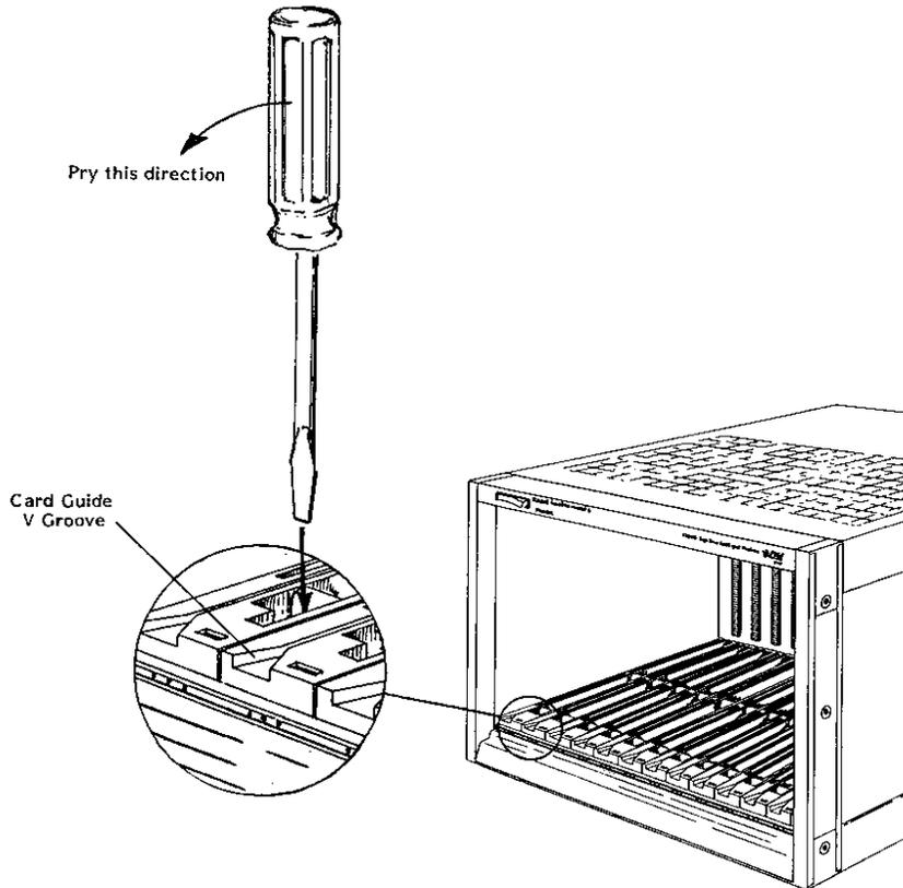
**Figure 5-2, Card Guide Removal and Replacement**
