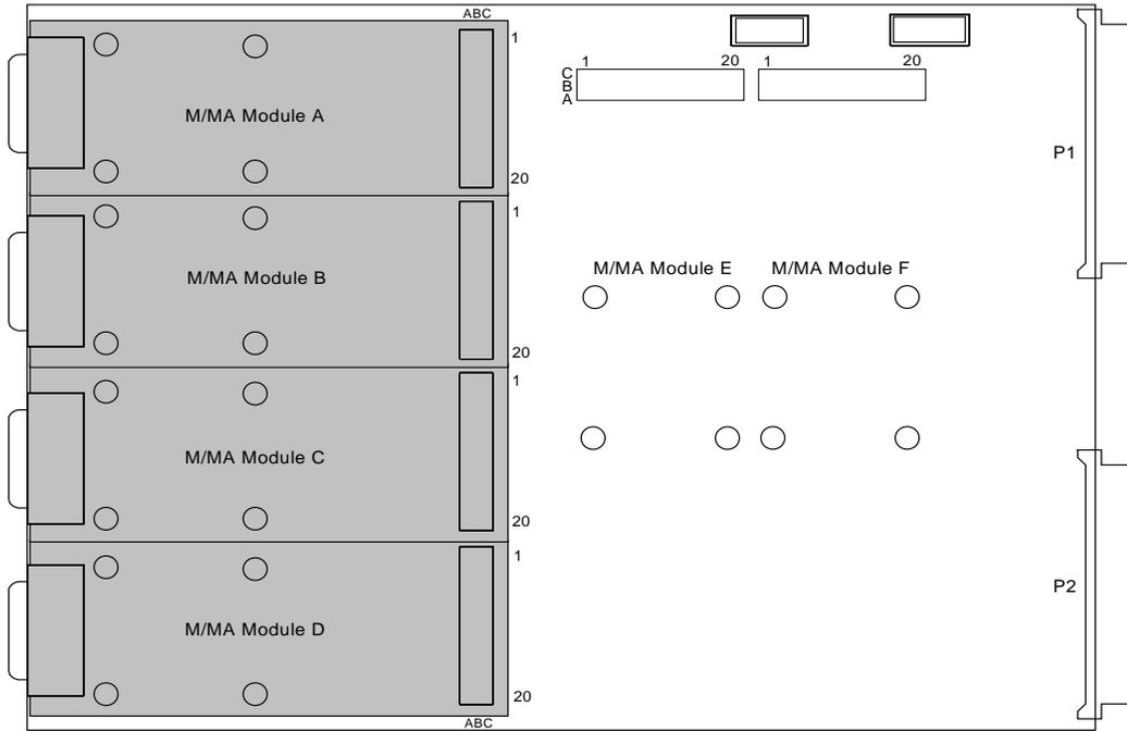
CONFIGURATION FOR FIVE (5) M/MA MODULES WITH FRONT PANEL ACCESS
