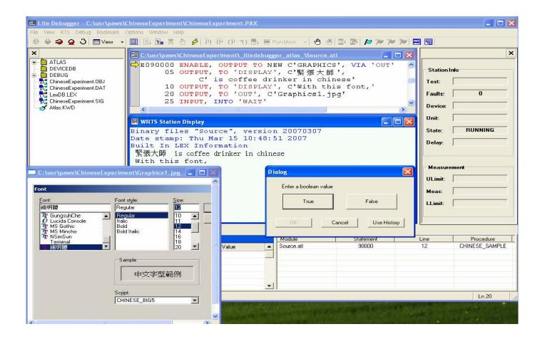
Example above displays the LiteDebugger debugging an ATLAS source program containing Tradition Chinese messages. It also displays the WRTS Station Display showing the traditional Chinese characters as a result of the OUTPUT, TO 'DISPLAY' ATLAS code.
