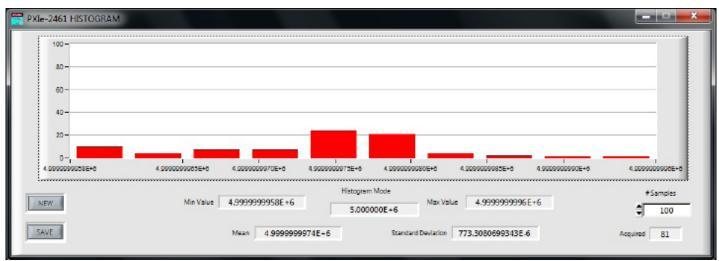
Figure 3: PXIe-2461 Histogram Characterizing a 5 MHz Oscillator Over a Pre-Determined Number of Samples
