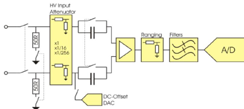
Front-end block diagram of a pair 6084-2105 channels
