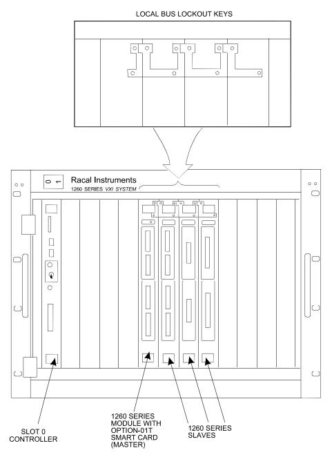
Figure 1-7, Local bus Key Installation
