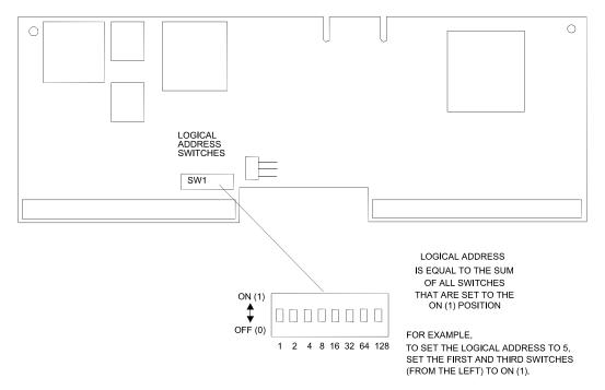
Figure 1-2, Setting the Option-01T Logical Address
