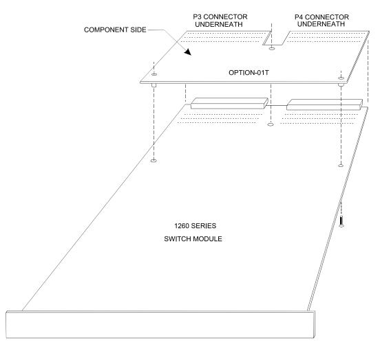
Figure 1-1, Installing the Option-01T
