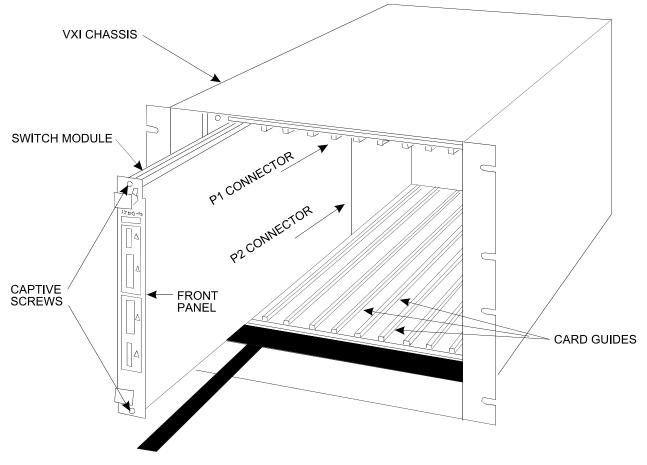
Figure 1-8, Switch Module Installation
