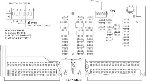
Figure 1-3, Local Bus Jumper Switches and Module Address Switches
