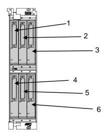
Figure 3-1, Front-View – Module Addresses for 1 through 6
