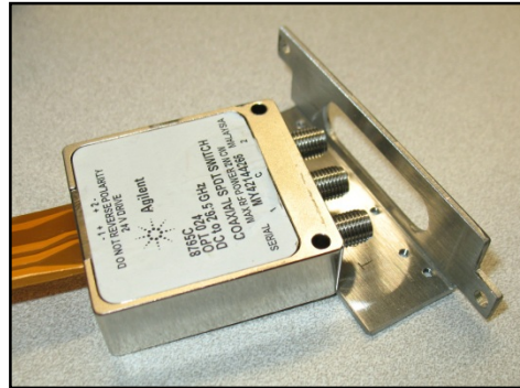
Figure B-3, Matching the Switch Mounting Plate (Appearance Typical)
