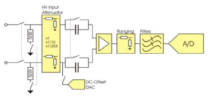
Front-end block diagram of a pair 6084-2105 channels
